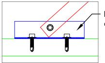
Field locate to center of strut intersection.
