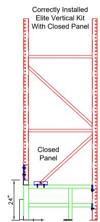
Cut the factory diagonal strut to length for reconnection above repair kit. Fasten to repair kit using (1) Reconnection Angle or Channel and (2) <sup>3</sup>/<sub>8</sub>" diameter Tek screws. Connect strut to reconnection component with supplied fasteners. (All required components are included)
