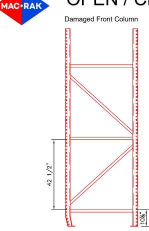
Determine which struts fall below the top horizontal of repair kit. Remove all those struts except for the factory diagonal that intersects with the top horizontal strut on the kit. Measure the intersecting point of diagonal strut and cut at that point. (Follow installation manual for complete Elite installation instructions)
